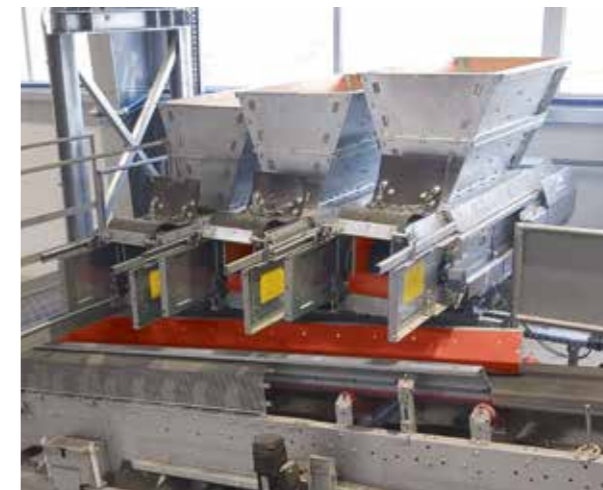
Color-Mix shuttle belt system
